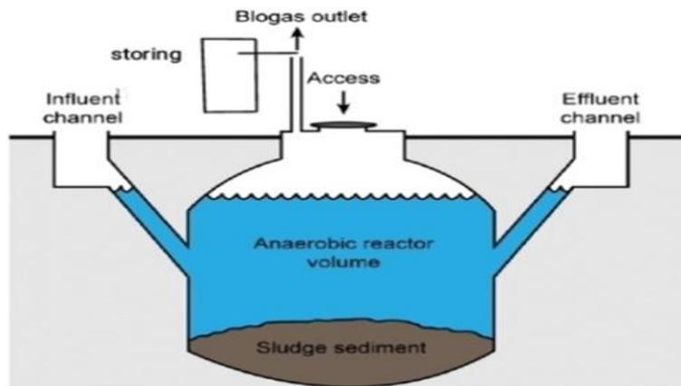
**Figure 3:** Biogas Plant
