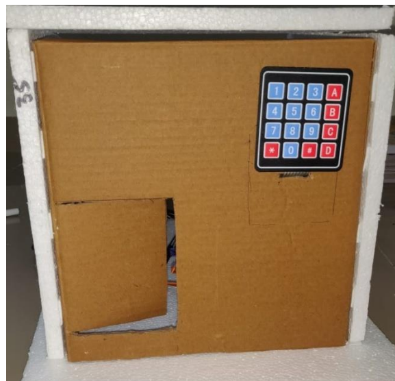
Figure 9: Unlocked status of the door
