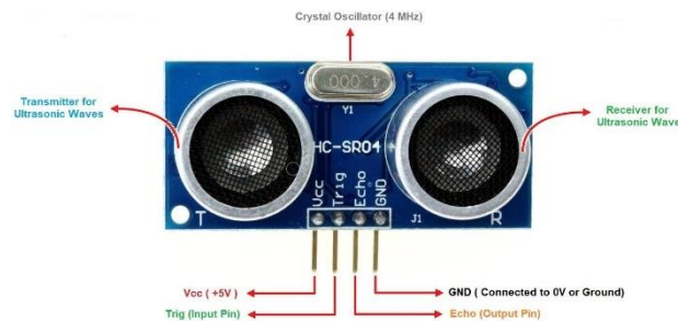
Figure 5: HC-SR04 Ultrasonic Distance Sensor
