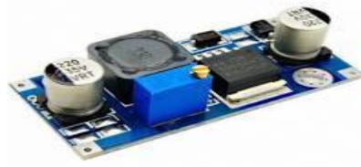
Figure 4. Lm2596 dc-dc Buk converter
