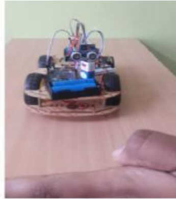
Fig 4.16 : Bot moves backward until it detects obstacle
