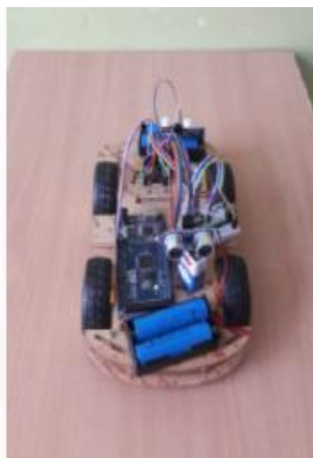
Fig 4.14 : Bot moves forward until it detects obstacle
