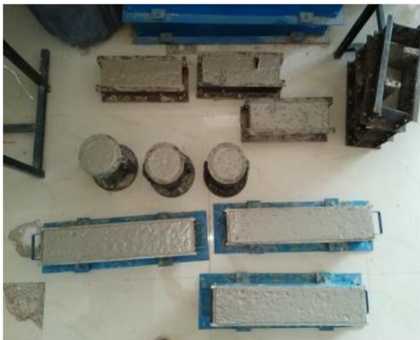
Figure 1:- Casting of Specimen
