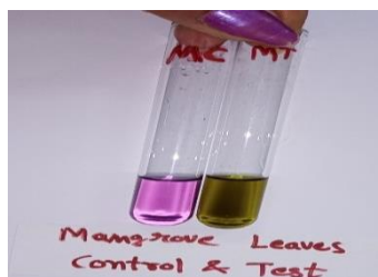
Figure 1: DPPH radical scavenging activity observed by change in the colour from purple (control) to yellow (Test).
