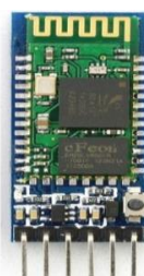
Fig.4: Bluetooth model HC05
