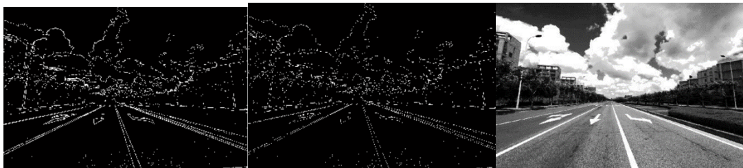
Figure 3: (a) 3x3 Bilateral Filter (b) Followed by SL | SR (c) Refined (Filtered) Picture
