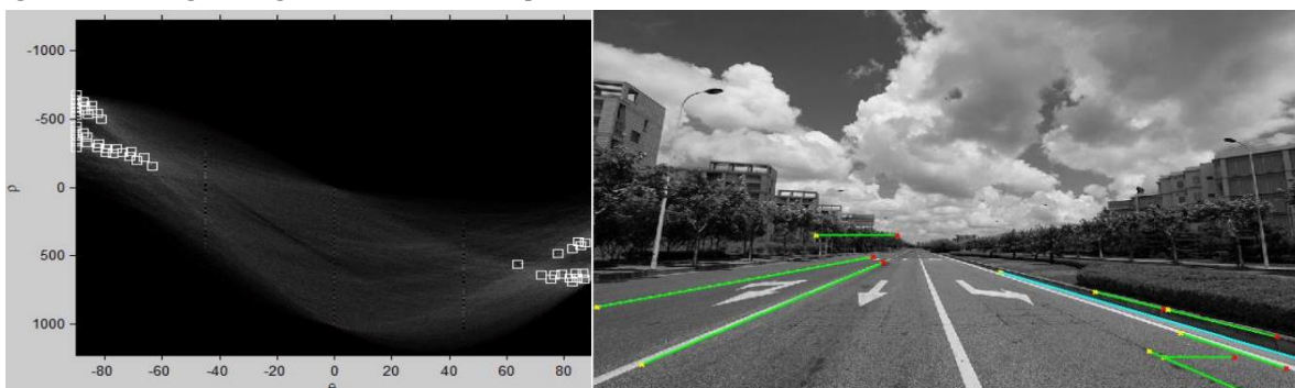
Figure 5: (a) Identification of Hough Lines (b) Obtained results
