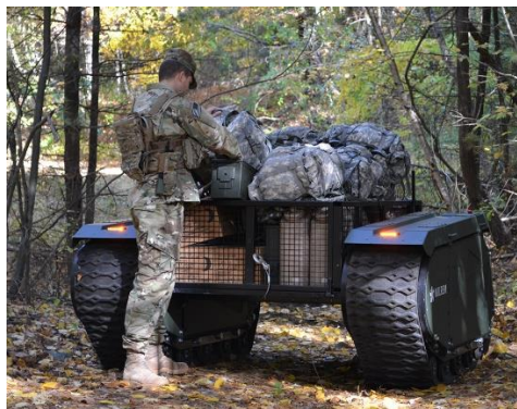
Fig.10. The Titan unmanned modular ground vehicle developed by QinetiQ North America and Milrem Robotics.
