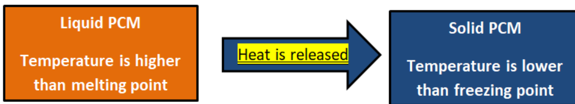
FIG.2 THE HEATING EFFECT OF PCMS
