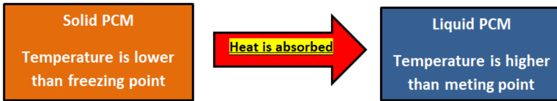
Fig.1 THE COOLING EFFECT OF PCM
