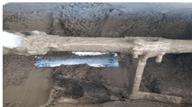
Fig :- Mixture Between Blades Are Not Mixed In Concrete Mixture Machine
