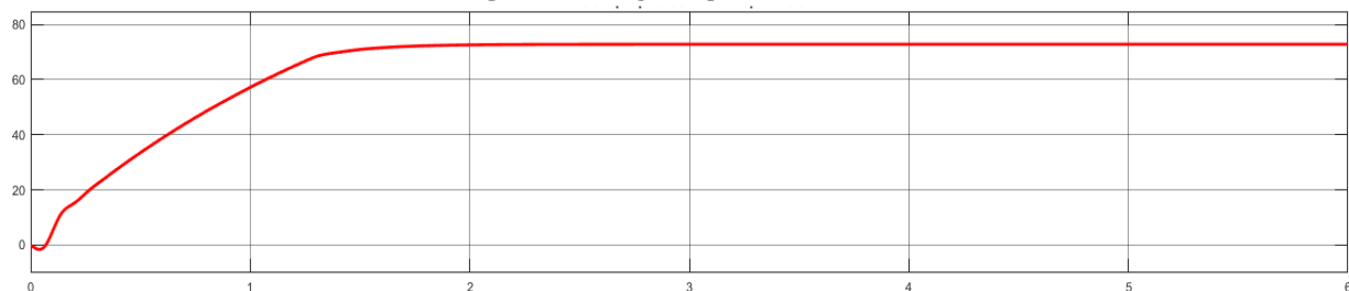
Figure 1.9 Motor speed at rated load
