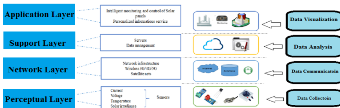
Figure 2: Different Layers of the Solar PV IoT based monitoring systems.
