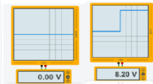
Fig.13 Output Waveform and Voltages of motor Turn ON
