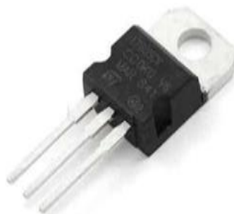
Fig.8 Voltage Regulator LM7805
