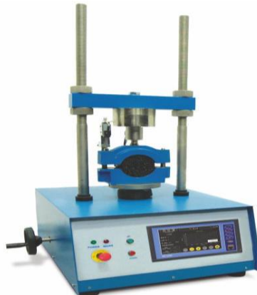
Fig-9: Marshall stability test
