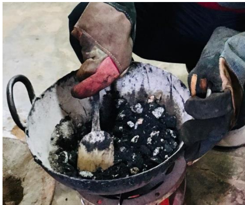
Fig-7: Mixing of bitumen
