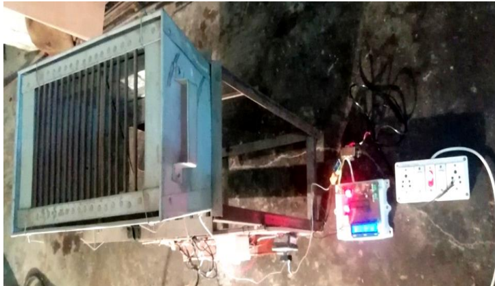
Figure.2 Experimental setup with digital temperature controller device
