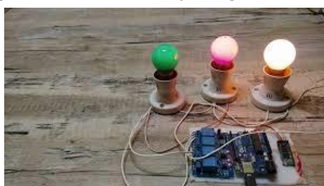
Fig 7. Hardware Implementation of Home Automation System
