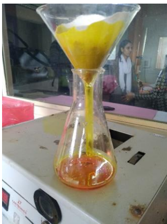
Fig no-2 (extraction of curcuminoids by filtration)
