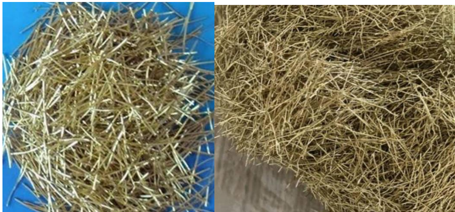
Pic :- Micro steel fiber
