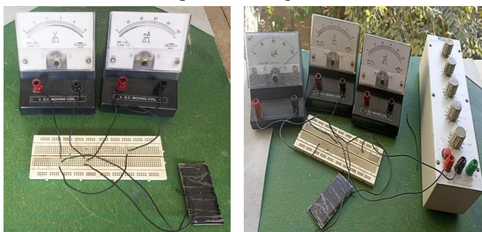
Figure 2: Experimental arrangement to study characteristics of solar panel a) without load resistance b) with load resistance.
