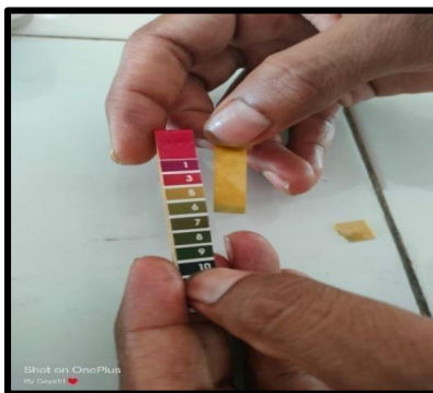
Figure 7: pH Determination of cream
