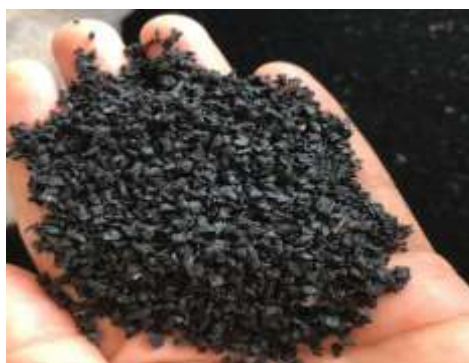
Figure 5: Crumb Rubber (Fine Aggregate)
