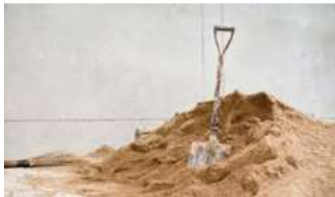
Figure 4: Fine Aggregate (Sand)
