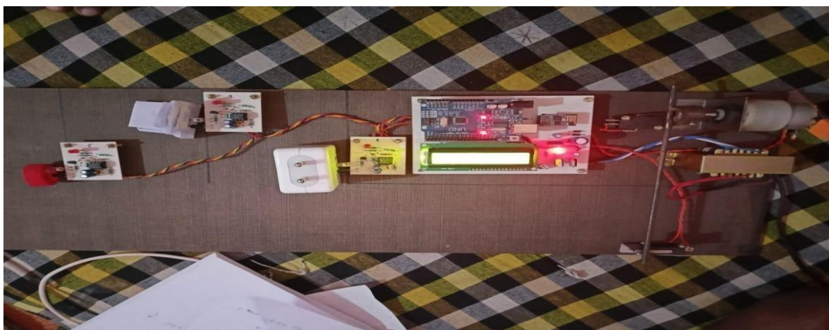
Gate is closed when all the slots are full and LCD will show the status of Slots which are full.
