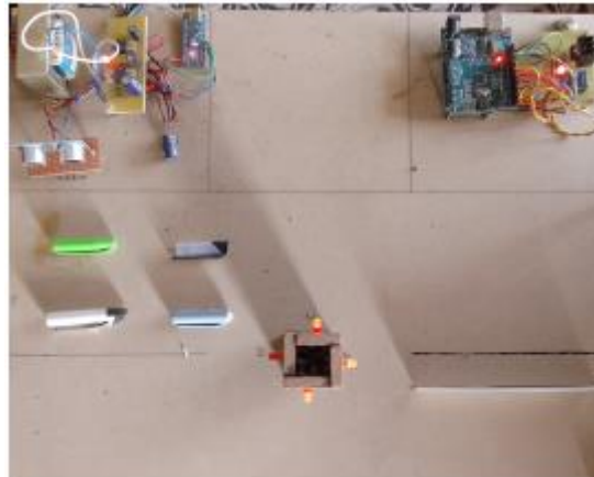
Figure 10: When Traffic is detected the divider is extended
