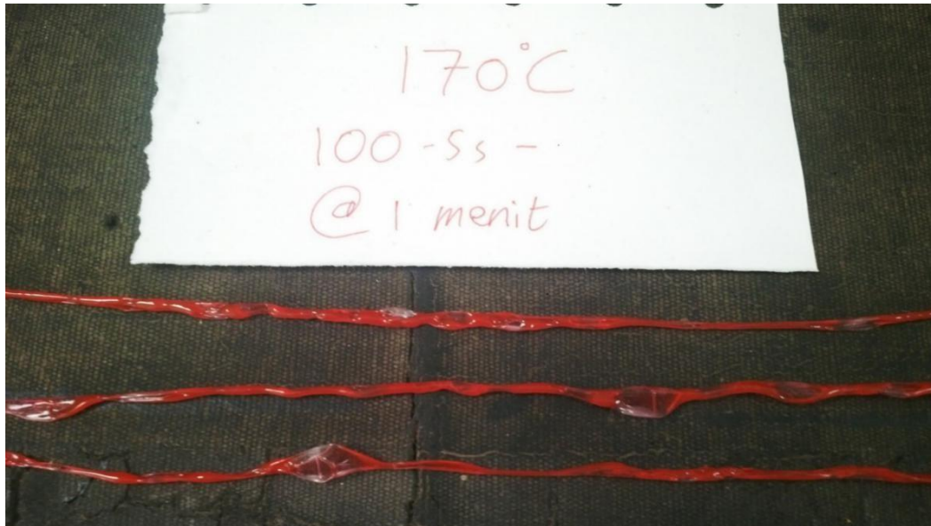
Figure 3: Results of extruded filaments with a heating temperature setting of 170°C and screw speed of 100 (12 RPM)
