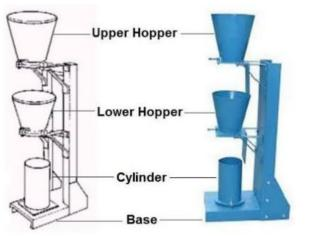
The compacting factor test is intended for use primarily in laboratories, but it can also be used in the field. It is more precise and sensitive than the slump test and is especially useful for very low-workability concrete mixes. It istypically used when concrete is to be compacted by vibration.
