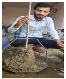
The slump cone test is a simple and effective method for assessing the workability of fresh concrete in India, and it is widely used in the construction industry to ensure that the concrete is suitable for its intended purpose
