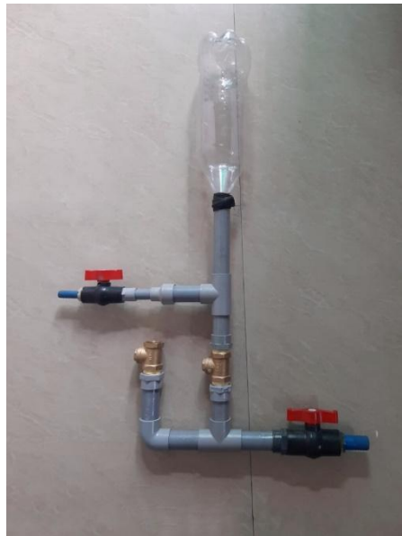
Figure 2.2: Actual model of ram pump used
