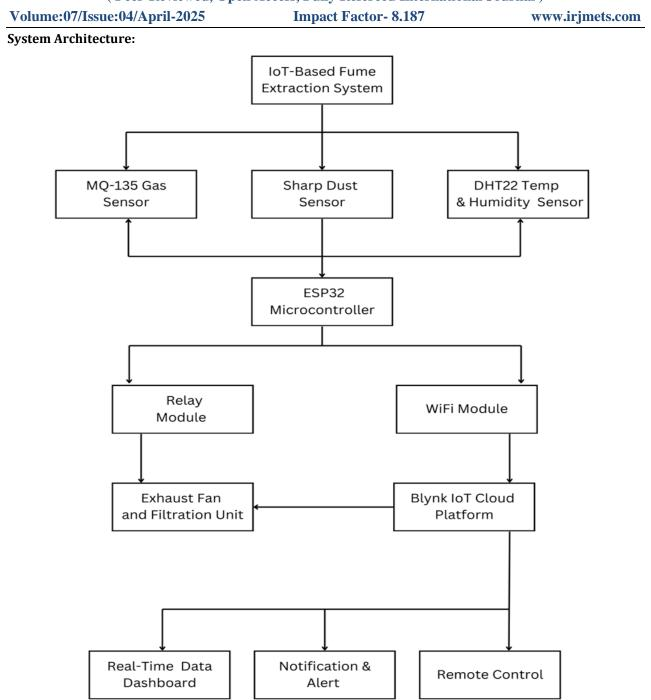
The IoT-Based Fume Extraction System architecture integrates environmental sensors (MQ-135, Sharp Dust, and DHT22) with an ESP32 microcontroller for real-time monitoring. Data is transmitted via a WiFi module to the Blynk IoT Cloud Platform, enabling remote control, alerts, and dashboard visualization, while controlling the exhaust and filtration unit through a relay module.
