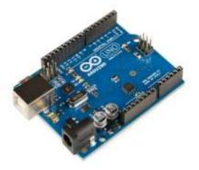
Arduino Uno is an 8-bit ATmega328P microcontroller. To support the microcontroller, it uses the components such as crystal oscillator, serial communication, voltage regulator, etc. It has 14 digital I/O pins( 6 pins can be used as PWM pins). It has six separate analog input pins, a USB connection, a Power barrel jack, an ICSP header, and a reset button.
