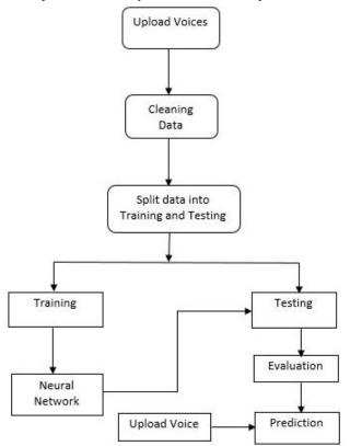
The above architecture ensures a structured and efficient workflow, enabling robust speaker recognition using deep networks. It effectively combines data preprocessing, neural network training, and real-time prediction for secure and accurate voiceprint authentication.
