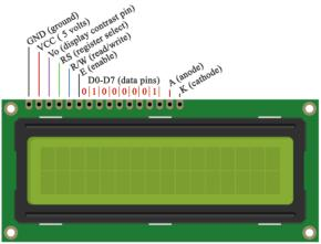
There are two lines of 16 characters each, which is what a 16x2 LCD can display. Each character is shown in a 5x7 pixel matrix on this LCD. Command and Data are the two registers on this LCD.
