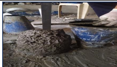
Figure 10: Slump Cone Test
