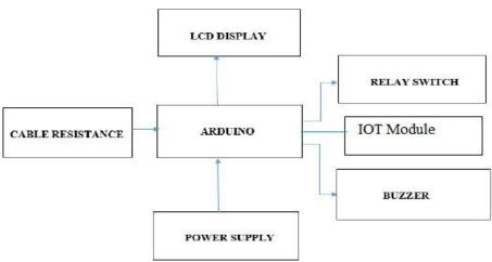
Fig 1: Block Diagram of system
