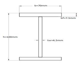
Figure 2: Dimension of original section
