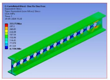
Figure 7: Equivalent Stress
