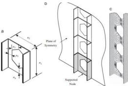
Figure 1: Sample finite element mesh and controlling parameters for analyzed castellated
