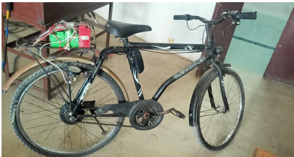
Fig 2: Prototype of self chargeable E-Bicycle using Dynamo
