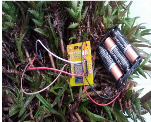
Figure 6: Soil Monitoring System Prototype.
