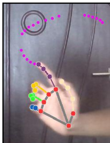
Figure 13: Algorithm tracking the index finger of the hand using Mediapipe
