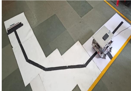
Figure 6: A.G.V. lifting on the marker.
