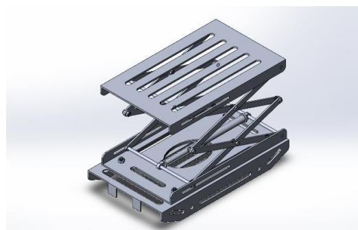
Figure 1: 3D Model of A.G.V.
