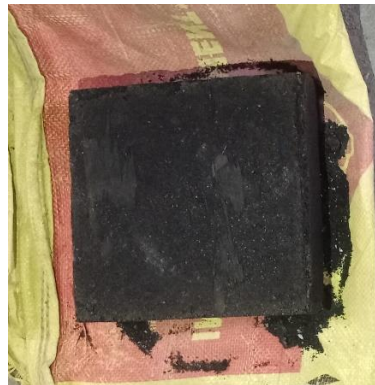
Fig. 3.1 plastic paver block
