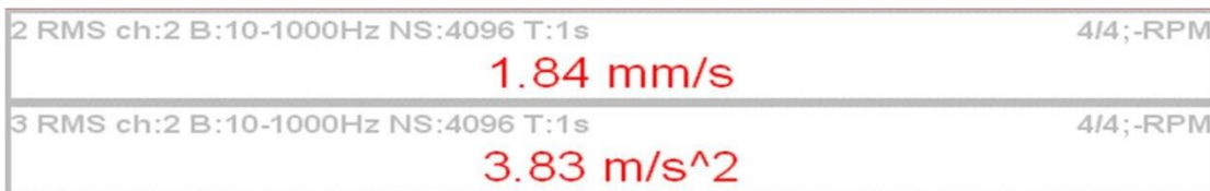
Figure 9: Velocity and Acceleration for 15Kg load at 1100 RPM
