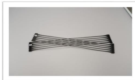
Fig 7: Uniaxially Stretched Geogrid
