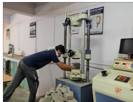
Fig 2: Testing of cube
