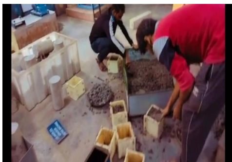
Fig 1: Casting of cube
