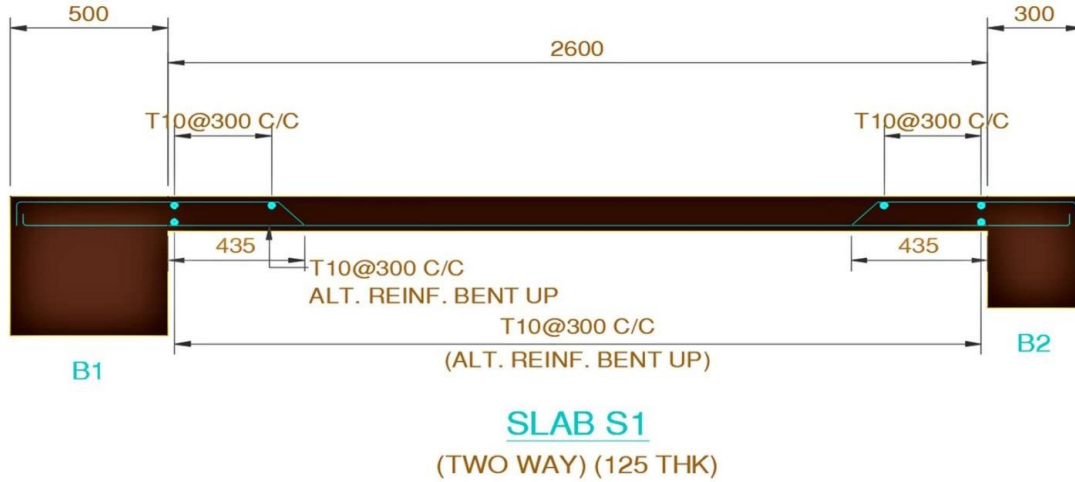
Figure 11: Sectional details of a slab
