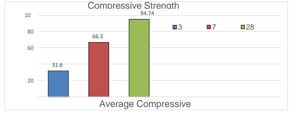
Average compressive strength of recycled aggregates at 3, 7, 28 days
