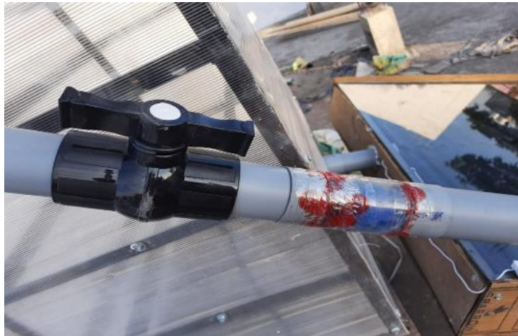
Fig: Regulate valve for recirculation exhaust hot air with breather for remove moisture
