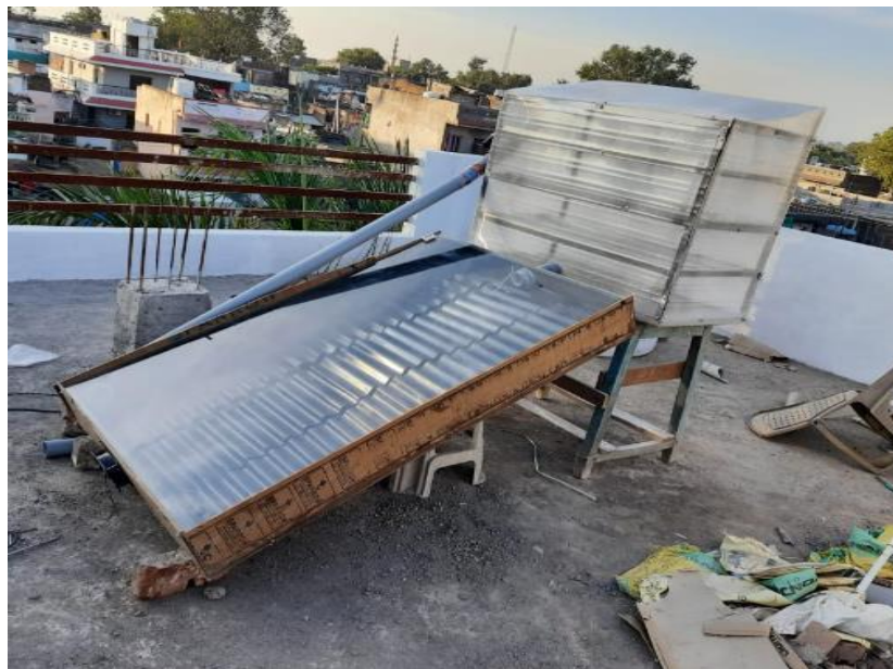
Solar dryer with recirculation duct arrangement
