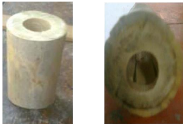
* Compression test specimen from internode region before and after the test *
