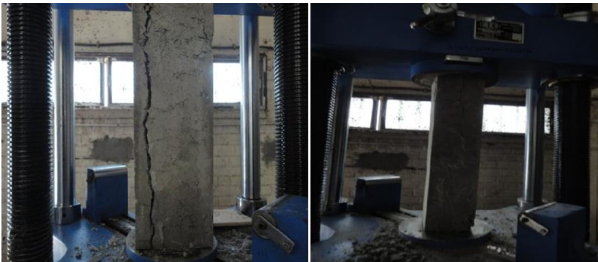
Fig. 2- Failure of rectangular bamboo reinforce concrete column.
