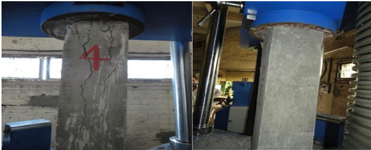
Fig. 3- Failure of square bamboo reinforce concrete column
