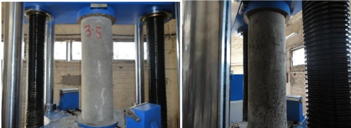
Fig. 1- Compression test on circular bamboo reinforce concrete column
