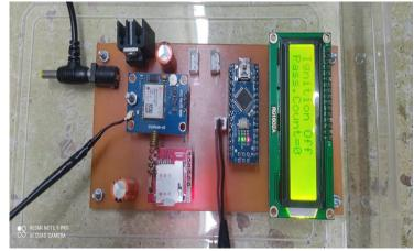
This shows the output of our project. and shows count of passengers which is increasing one by one.as well as the status of ignition.
