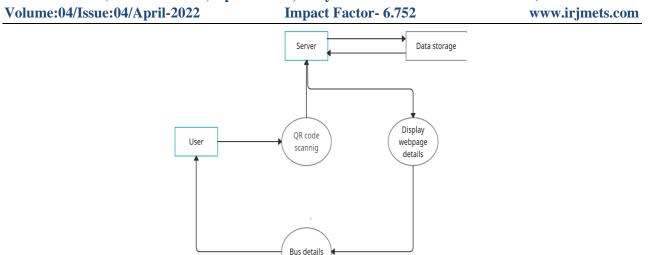
This is the Data flow diagram of our project, first user scans the QR code after that request sends to the server access the data from cloud then the server displays the whole details of bus, that is route of the bus, real time location of bus, bus number and exact count the number of passenger in bus.
