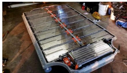
Figure 9: Tesla Model S Battery Pack.
