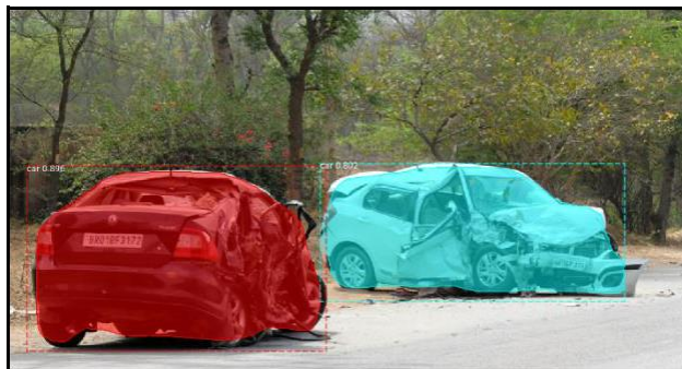
Fig 2: Results of Accident Detection using mask rcnn
